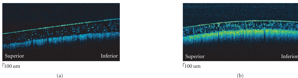
FIGURE 7: Comparison between OCT tomograms of Japanese porcelain (a) and faience (b).
